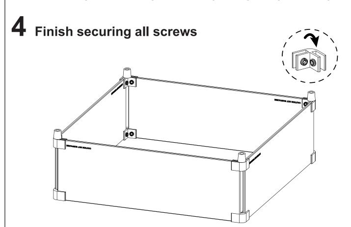
Gently secure all screws (on all brackets) 1/4" to 1/2" turn until panels are secure. DO NOT OVERTIGHTEN.
