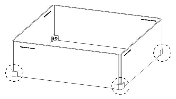
DO NOT overtighten screws. Tighten until snug. Overtightening can break glass.
