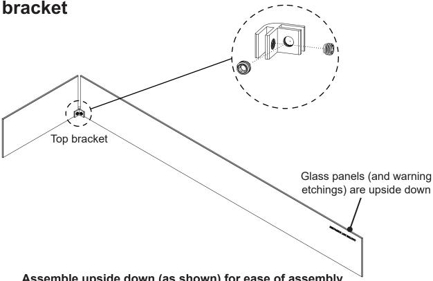
Assemble upside down (as shown) for ease of assembly.
