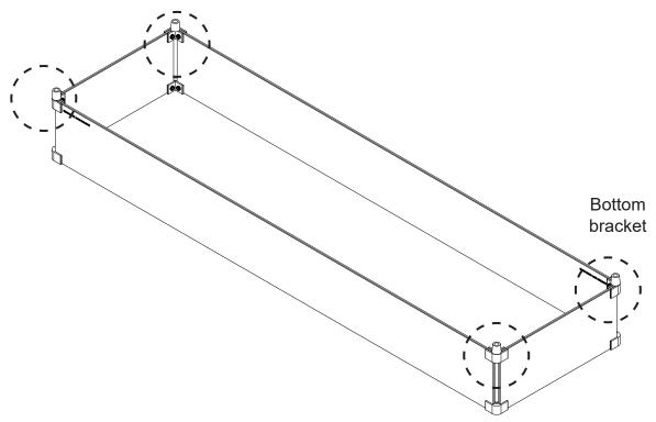
DO NOT overtighten screws. Tighten until snug. Overtightening can break glass.
