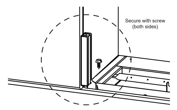
Secure brackets using provided hex screws and a <sup>5</sup>/16" nut driver (both sides).
