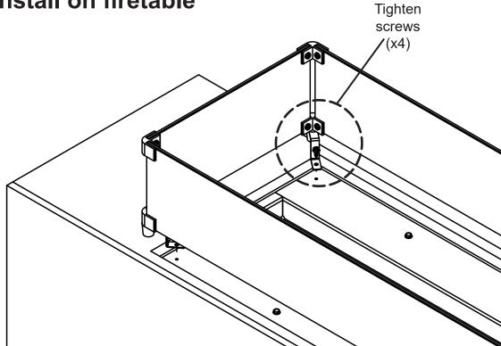
Use a  $^{5}$ /16" nut driver and supplied four screws to fasten guard in place. Start all four screws to ensure guard is properly aligned, then fasten all screws.
