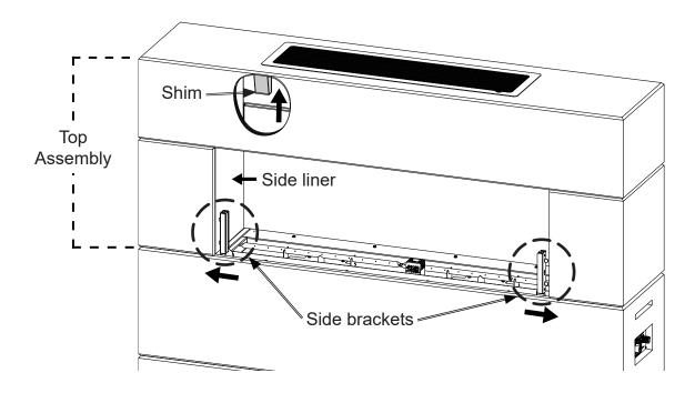
Temporarily loosen shims to insert side brackets between side liners and top assembly.
