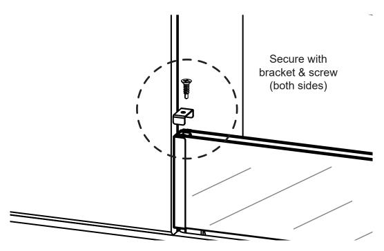
Place a top bracket, then secure using a provided screw and a small-sized Phillips screwdriver. Repeat for second top bracket.
